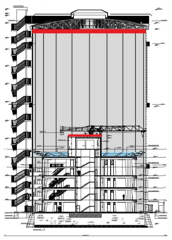
Within the Visiodrome, the projectors can be installed at the points marked in red. Requirements: No glare on the circular grandstands (light blue areas). Minimal shadows cast on the surface. The projectors must be easily accessible for maintenance and corrections. The optics of the devices must be aligned with the positions.
